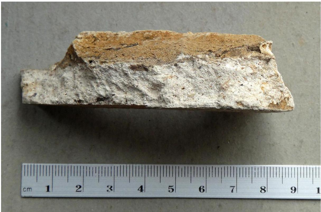
Edge of plaster fragment, showing it was applied in two layers of different composition.
